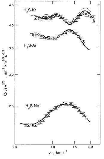
FIG. 1. Absolute integral cross section Q for the scattering of H<sub>2</sub>S by Ne, Ar, and Kr, as measured as a function of the H<sub>2</sub>S molecular beam velocity v and plotted as  $Q(v) \times v^{2/5}$  (see text). Curves are calculated from best-fit interaction potentials of Fig. 2 and Table I. In the case of H<sub>2</sub>S-Kr the dashed line is the cross section calculated without correction for the experimental angular resolution (see text).
